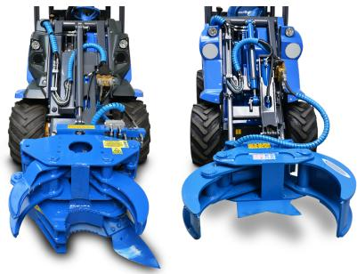
Two models are available: with fixed blade for trunk up to 10 cm diameter and with hydraulic blade for trunk up to 15 cm diameter. Through the reach of the MultiOne's boom, this unit can also be used to prune branches, and clear scrub growth in difficult to reach places.
