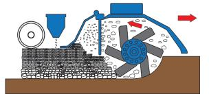
the rear field roller. With the optional seeding unit you are able to make a ready lawn surface on one pass. Stone burier is most commonly used when the topsoil needs to be milled thoroughly.
