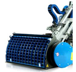
bucket is emptied from the bottom hatch. Hatch opening is powered by a hydraulic cylinder controlled from driver's seat. The bucket is also equipped with a flexible emptying tube which mounts on the bottom hatch. This enables pouring of the concrete further away from the bucket. Designed for high volume production, this unit minimizes downtime.
